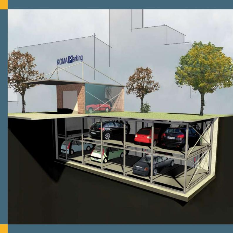
An automatic system for independent parking, based on pallet transfers horizontally (all pallets together) and vertically (pallets are lifted by both sides with a lifting device). A single area is shared for both arrival and departure, clear at most times. It can be enhanced with a turntable. For indoor use only. The systems can be above ground, under ground, and combined.
