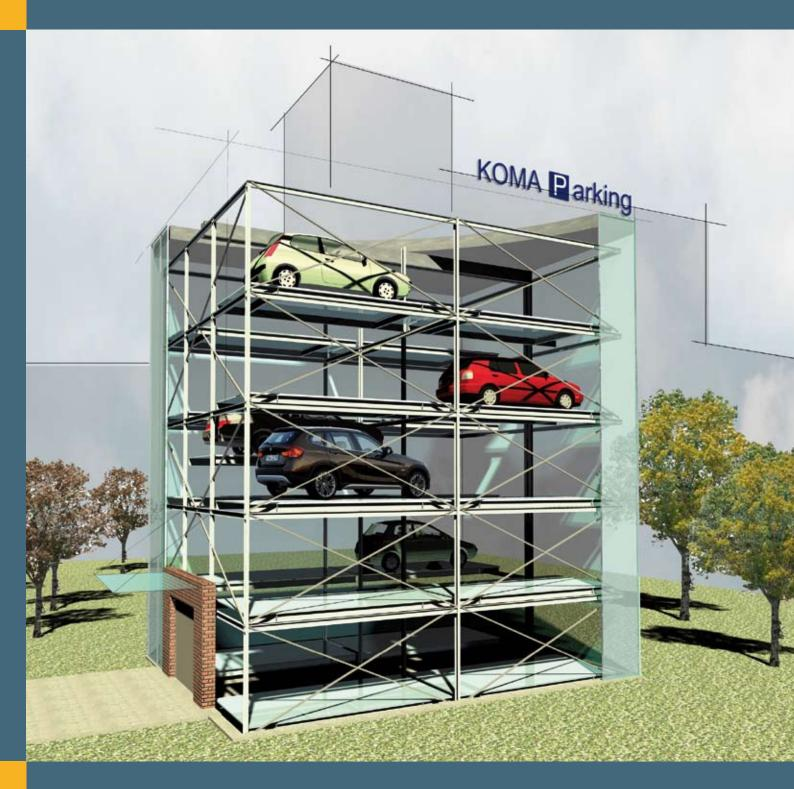
An automatic system for independent parking, based on stacking cars and shifting pallets to either side of the lift with skips. It is a parking design with a huge capacity, featuring multiple lifts, clearing slots and skips.
